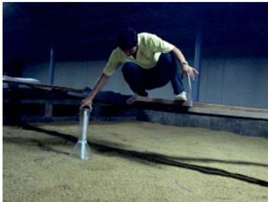
Figure 4. Checking the air distribution.
