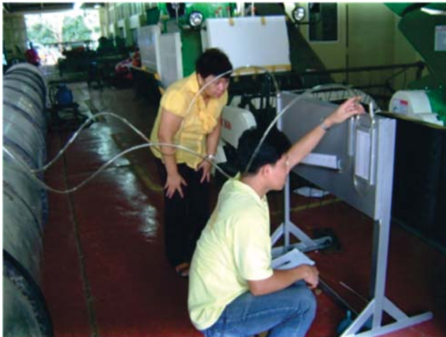
Figure 5. Static pressure measurement using an inclined manometer.
