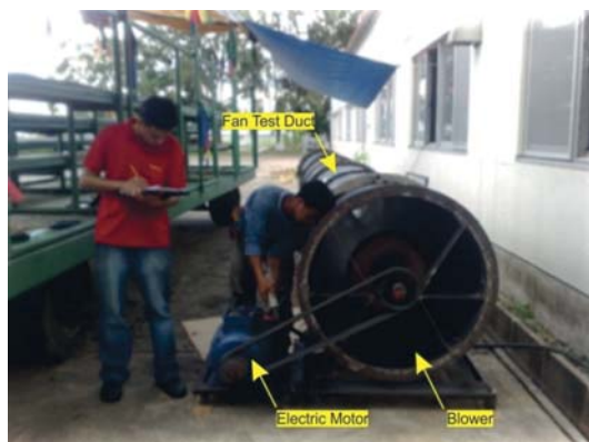
Figure 6. Measurement of power consumption of the blower using a power meter.
