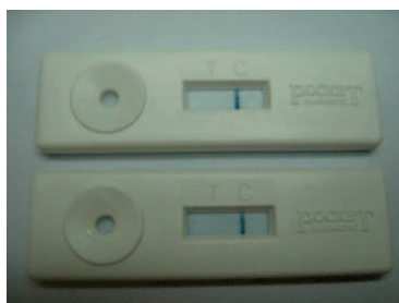
Figure 4. R. solanacearum test kit showing a negative test.
