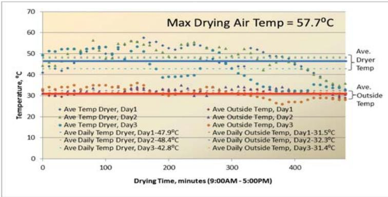
Figure 3. Performance of the fabricated solar dryer without the heat collectors.
