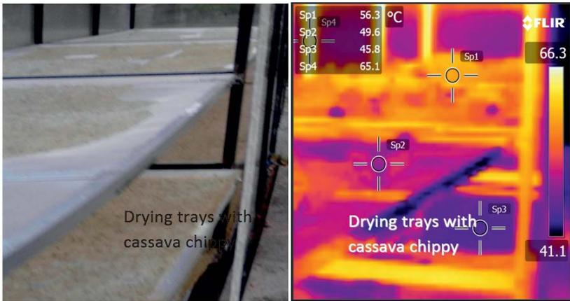
Figure 7. Temperature distribution of the inside of the drying chamber with wet cassava chippy being dried, using an infrared imaging camera with the heat collector.
